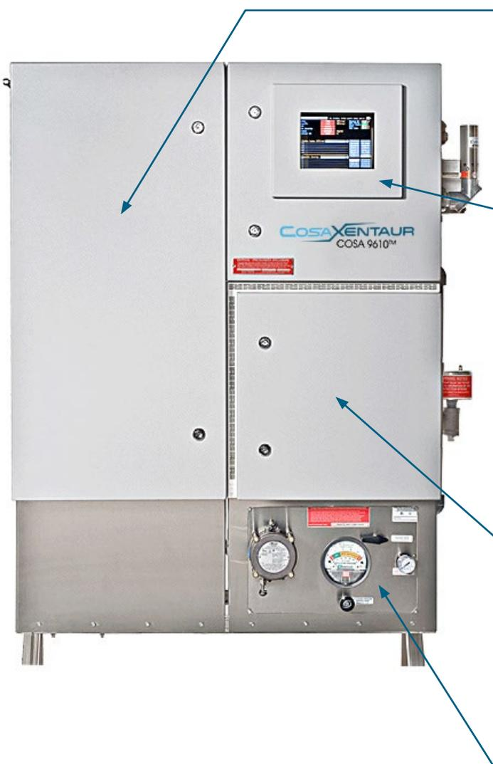
The **gas mixing compartment** contains sample conditioning and the gas mixing system. Components in this compartment are intrinsically safe. The gas mixing compartment can optionally be heated to avoid condensation of heavier gas constituents.
